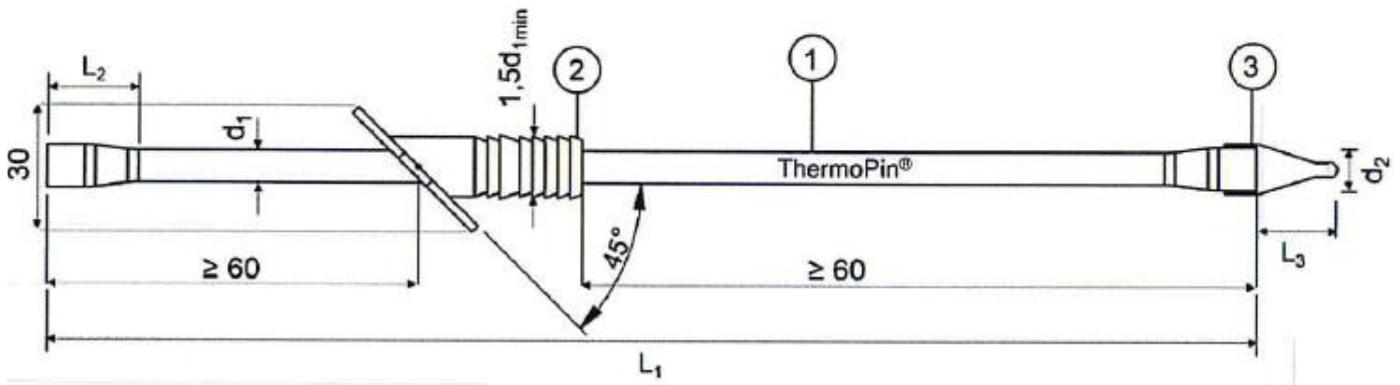
ThermoPin tie anchor Type D: GFK anchor with sloping plastic sleeve. Dimensions in [mm]
