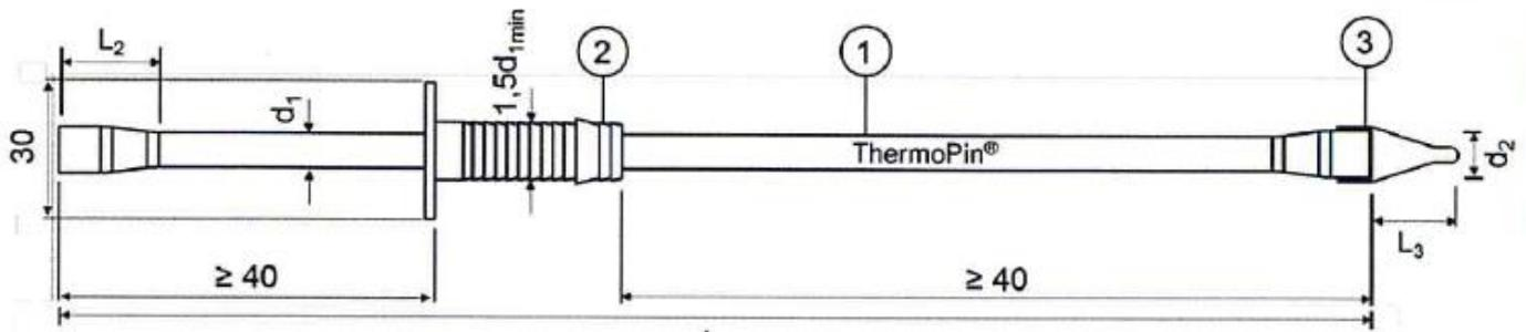
ThermoPin tie anchor Type H: GFK anchor with straight plastic sleeve. Dimensions in [mm]
